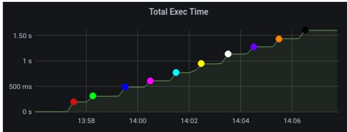
Figure 62: Latency to delete 1000 rules in total atop P4 topologies of increasing size.
