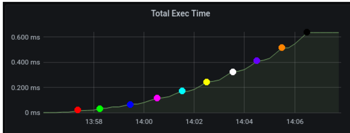
Figure 61: Latency to retrieve 1000 rules in total atop P4 topologies of increasing size.
