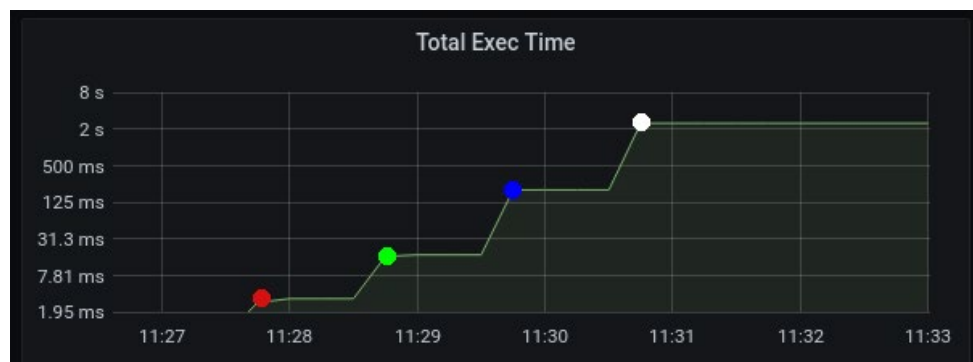
Figure 57: Latency to install P4 device configuration (SetConfig RPC) with exponentially increasing number of rules (1,10,100,1000).
