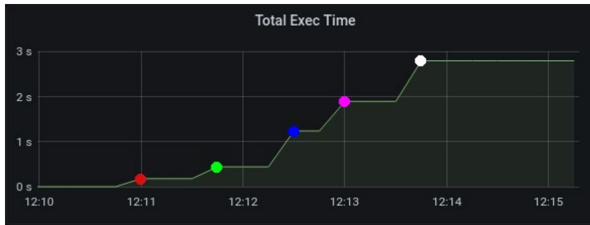
Figure 91: Latency to tear 1-5 L2NM services down atop pairs of P4 devices.
