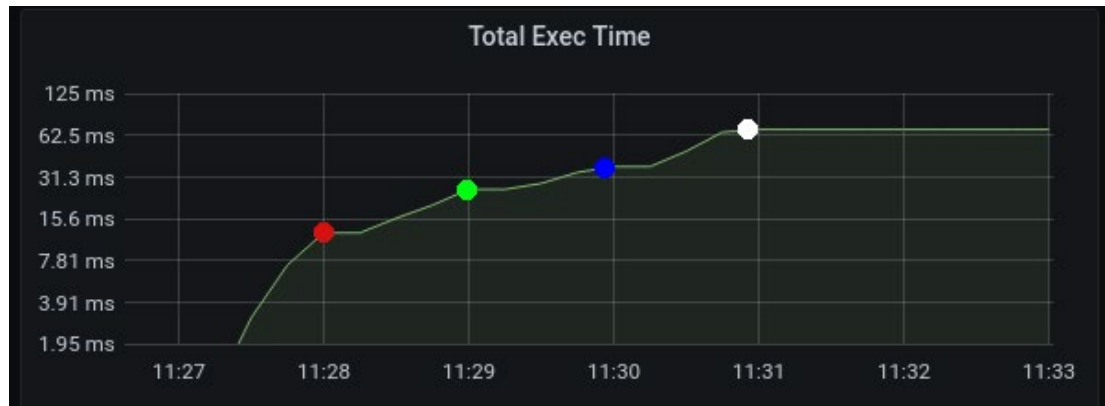
Figure 58: Latency to retrieve P4 device configuration (GetConfig RPC) with exponentially increasing number of rules (1,10,100,1000).
